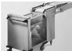
Flat belt clearing conveyor Dimensions W x H 500 x 900 mm
